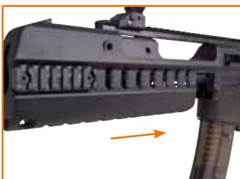
5. Carefully push the handguard back onto the weapon. Make sure that the position in the guide rail is correct.
