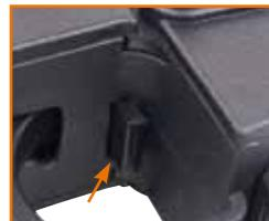
1. The hop-up is located in the bottom window of the sleeve ejection. Pull the tensioning lever back to get to the adjusting wheel of the hop-up.
