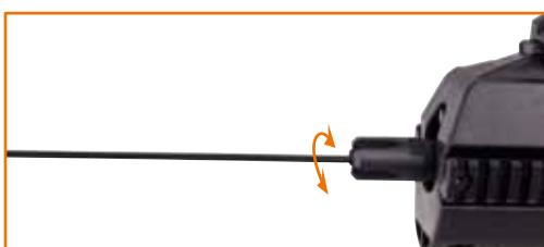
4. Introduce the end with the material strip into the barrel from the front with a rotational movement. To do this, remove the muzzle beforehand and expose the hop-up.
