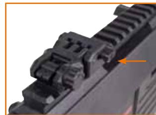
1. The sight can be flipped up with a push of the button. A button is located on each side of the sight.
